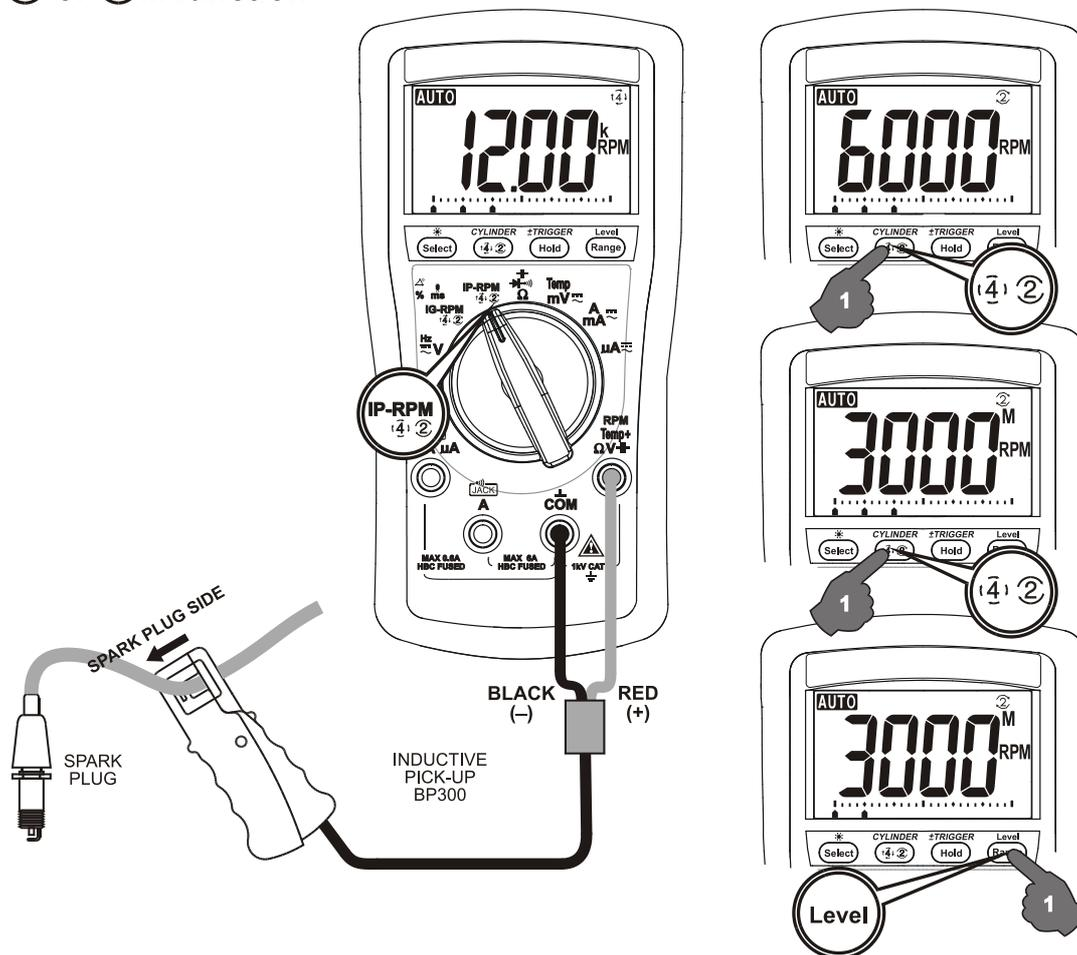
Press (4) (2) button momentarily to select through **RPM (4)** for 4-stroke, **RPM (2)** for 2-stroke and DIS, and **RPM (2) M** for special 2-stroke waste ignition engine
