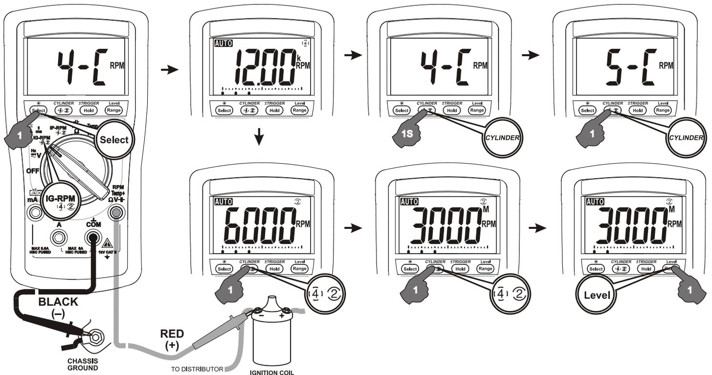
Press (4) (2) button momentarily to select through **RPM (4)** for 4-stroke, **RPM (2)** for 2-stroke and DIS, and **RPM (2) M** for special 2-stroke waste ignition engine
