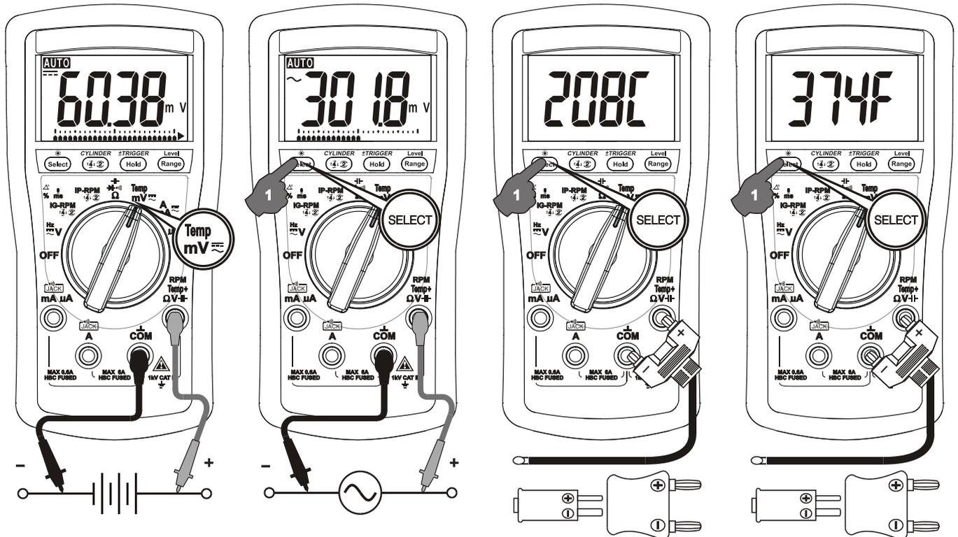
Note: Be sure to insert the banana plug K-type temperature bead probe Bkp60 with correct **+** **-** polarities. You can also use a plug adapter Bkb32 (Optional purchase) with banana pins to K-type socket to adapt other standard K type mini plug temperature probes.
